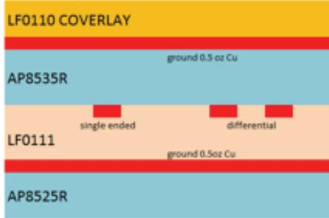
The above stackups were made to compare the performance of DuPont™ Pyralux® TK clad and bondply to the AP clad and LF bondply. The data in the next two graphs show data based on these two stripline designs.
