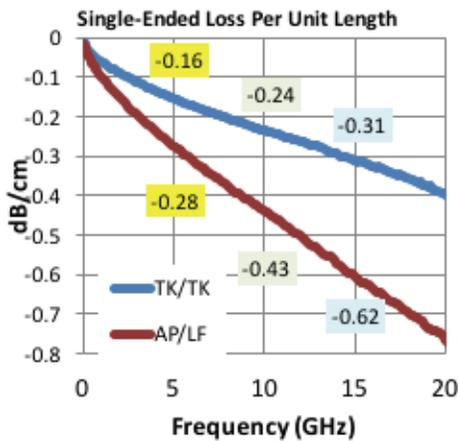
Graph above shows the loss in dB/cm up to 20 GHz. The TK constructions clearly shows much lower loss (dB is a log scale).
