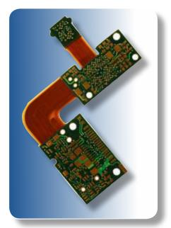
38N is an improved polyimide low-flow prepreg suitable for bonding multilayer polyimide rigid-flex, attaching heat sinks to polyimide MLBs, or other applications where minimal and uniform resin flow is required.
