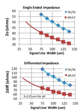
Graphs above show the impedance at different line widths for the two constructions. This shows the real advantage of lower Dk for making controlled impedance circuits. To achieve standard impedance targets at achievable line widths the AP/LF constructions would need to have a thicker dielectric between the two ground planes.
