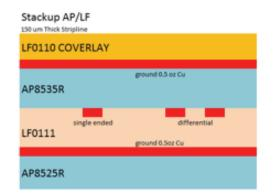
The above stackups were made to compare the performance of DuPont<sup>™</sup> Pyralux<sup>®</sup> TK clad and bondply to the AP clad and LF bondply. The data in the next two graphs show data based on these two stripline designs.
